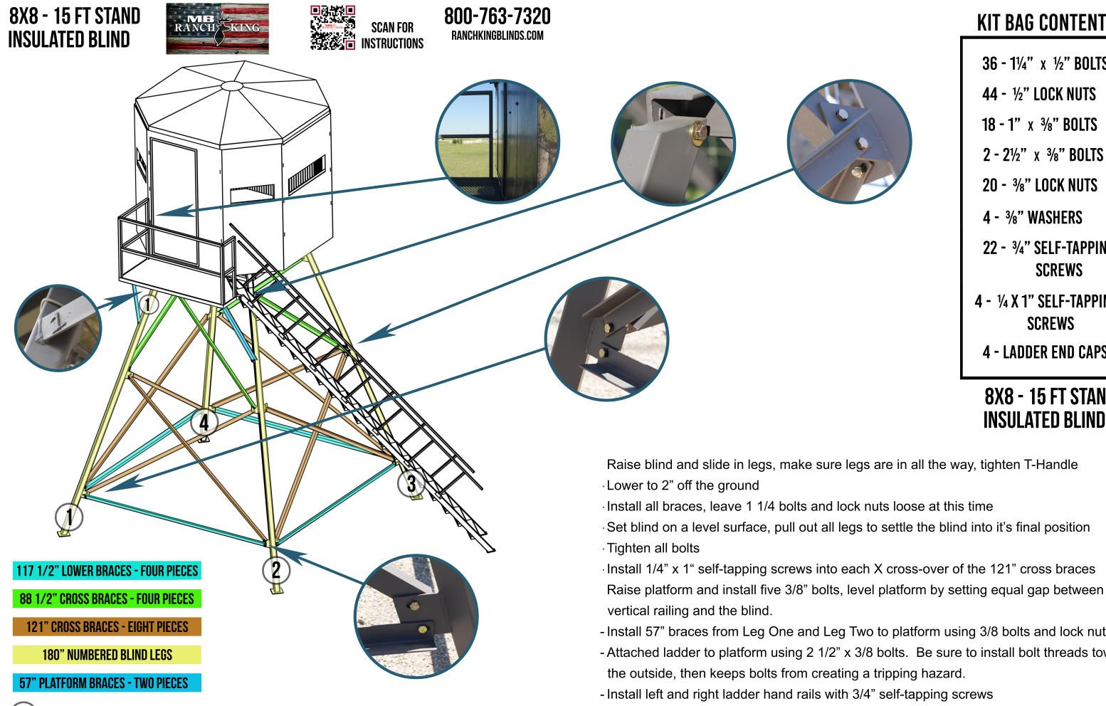
LEGS ARE MARKED AND INSTALLED WITH THE LEG NUMBER ON THE LEG AND BASE
