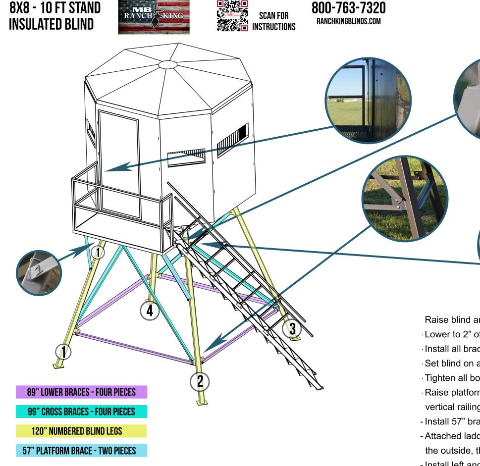
LEGS ARE MARKED AND INSTALLED WITH THE LEG NUMBER ON THE LEG AND BASE
