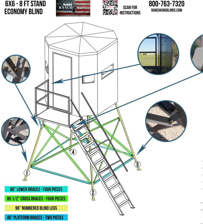
LEGS ARE MARKED AND INSTALLED WITH THE LEG NUMBER ON THE LEG AND BASE
