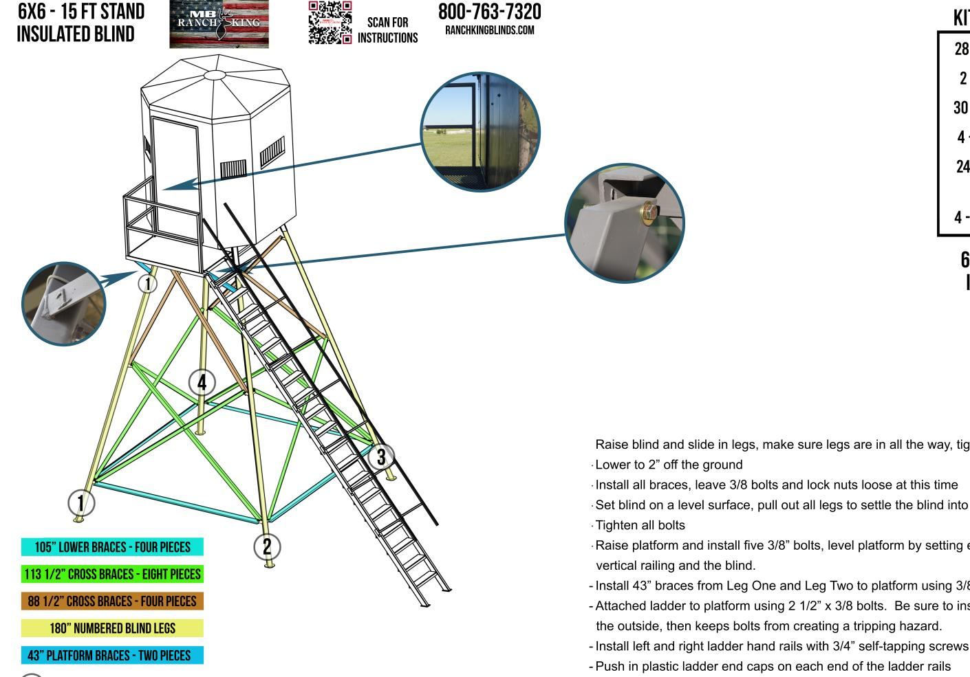
LEGS ARE MARKED AND INSTALLED WITH THE LEG NUMBER ON THE LEG AND BASE
