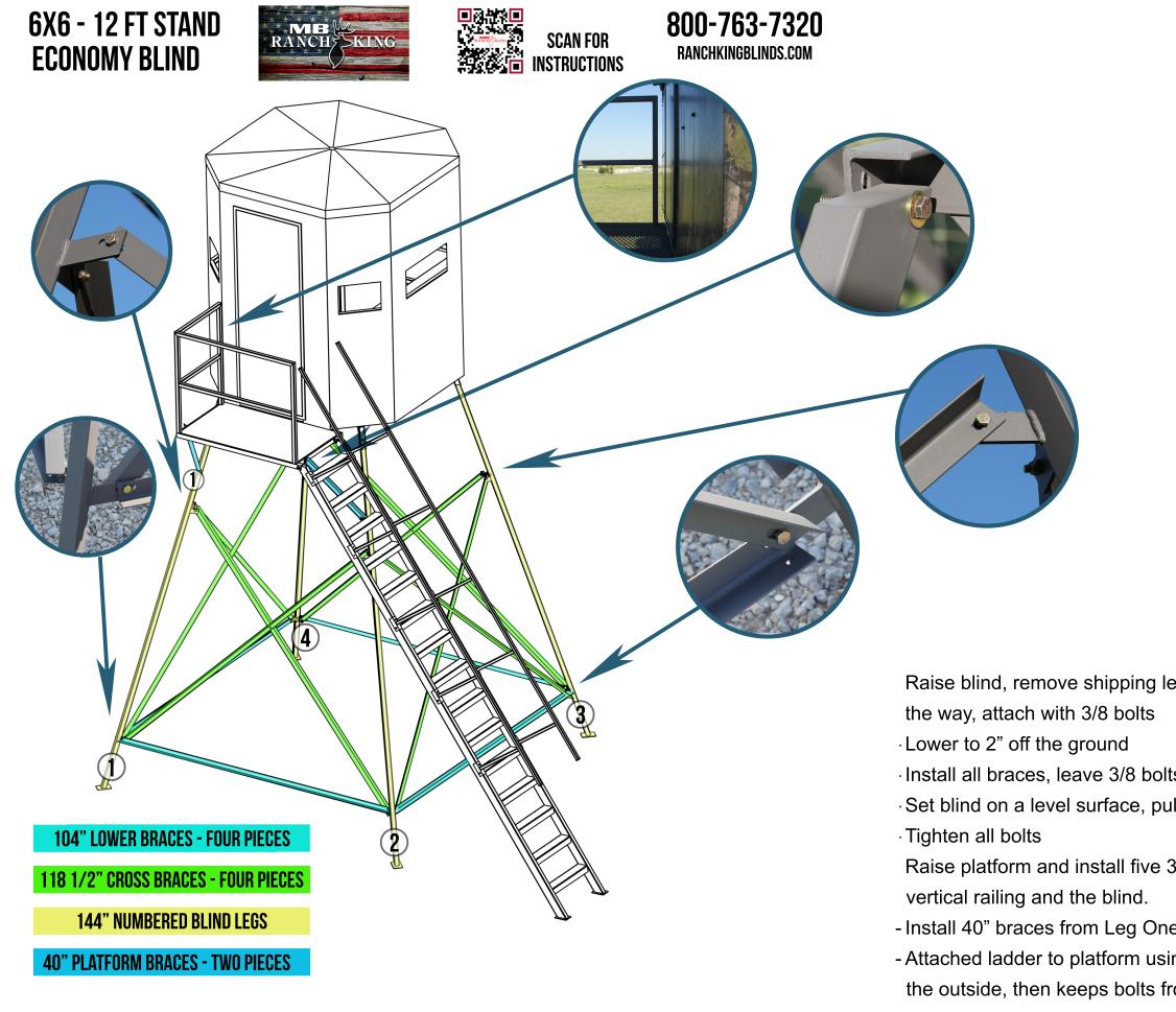
LEGS ARE MARKED AND INSTALLED WITH THE LEG NUMBER ON THE LEG AND BASE
